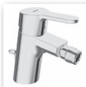
HANSAPRIMO one-hole single-lever mixer, DN 15 for bidet 4943 3203 chrome pop-up waste (metal), connection with flexible hoses G 3/8 projection: 107 mm
