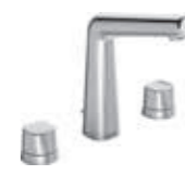
HANSADESIGNO trim kit concealed electronic mixer, DN 15 (G1/2) suitable for HANSA MATRIX installation unit 4492 2010* chrome with thermostatic temperature mixing device, sensory operation (infrared), incl. power supply and connection cable projection: 195 mm
