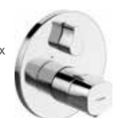
HANSALIVING trim kit with function unit thermostatic shower faucet, DN 15 (G 1/2) suitable for HANSABLUEBOX concealed unit 8113 9552* chrome with integrated ceramic volume regulation, function unit with service stops, without diverter
