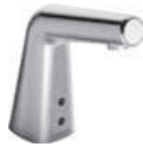
HANSADESIGNO electronic basin faucet, DN 15 mains supply 5193 2211 chrome incl. power supply and connection cable, MIKADO® Aerator, without pop-up waste, hygienic flush after 72 h for 30 sec at factory preset projection: 100 mm
