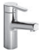
HANSADESIGNO one-hole single-lever basin mixer, DN 15 5172 2283 chrome without pop-up waste, HANSA 3S-Installation, connection with flexible pressure hoses projection: 119 mm
