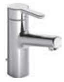
HANSADESIGNO one-hole single-lever basin mixer, DN 15 5191 1183 chrome pop-up waste (metal), HANSA 3S-Installation, connection using flexible hoses G3/8 projection: 119 mm
